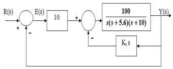
**b)** Using Mason's rule, find the transfer function, T(s) = Y(s) / R(s), for the system represented in the following Figure. [5 Marks]
